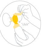
The membrane that provides overflow protection fits simply into the connector.
